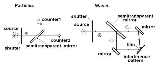
Fig. 1: Experiments with individual photons on semitransparent mirror
