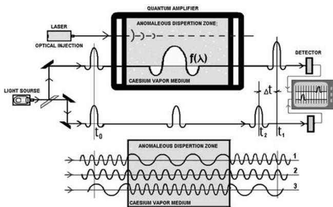
Fig. 5: Experiments of L. Wang - superluminal light propagation
